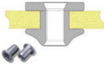
Placement of Threaded Fasteners
